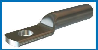
The increased barrel length ensures enhanced electrical and mechanical performance in heavy duty application. The absence of an inspection hole prevents the entry of water or moisture into crimped joints making them suitable for outdoor applications. The terminals are tin plated to avoid oxidization and to achieve maximum corrossion protection.
